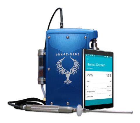
Overnight storage and calibration of the phx42 should be done indoors at or near room ambient conditions (15-25 °C or 59-77 °F) with a maximum humidity of 85%.
